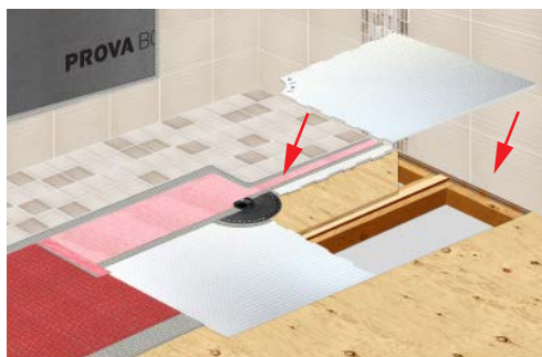
Complete Layered Curbless Installation
